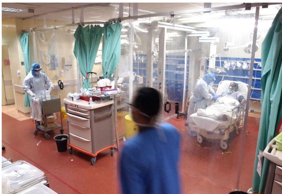
In Sungai Buloh Infectious Disease Hospital, Selangor, self-designated plastic sheet barriers were installed at patient treatment cubicles in Red Zone Emergency Department creating a makeshift isolated and safe treatment space. The hospital had enrolled the highest number of patients in Malaysia Photo credit: Abdul Razak Aziz
